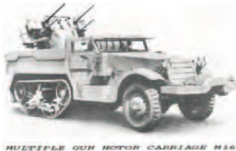
MULTIPLE GUN MOTOR CARRIAGE M16 ANTI AIRCRAFT
